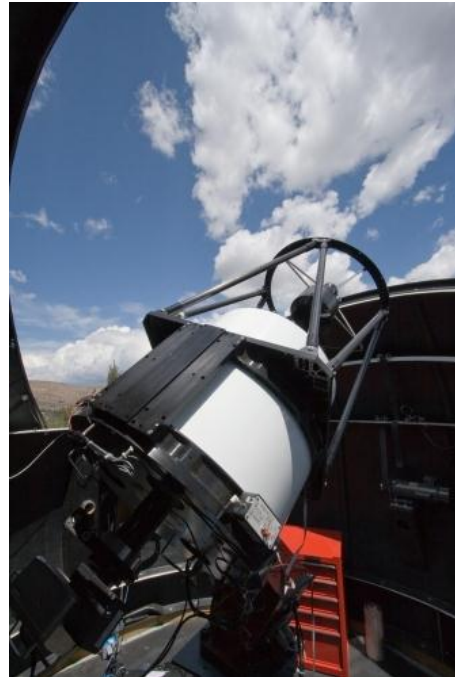
Figure 1. The .5 meter telescope at Blackbird Remote Observatory manufactured by RC Optical Systems.
